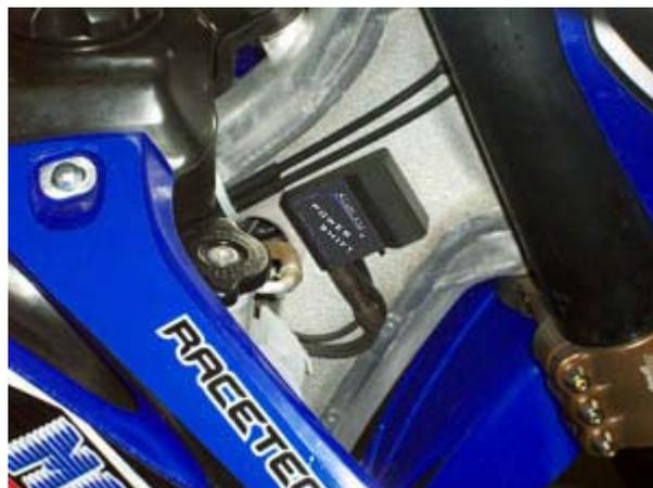
The small electronic control unit enables the user to set up the trip threshold and the cut off time.
